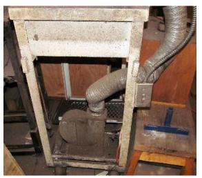
The manifold is a piece of box tubing with a couple of pipe sections that slide over the burners. Note the set screw at the rear. The connection to the flex pipe is through a slide gate. When first fired without the gate, the 3000 F refractory started to melt, so having the ability to choke off the flow is a good thing,
