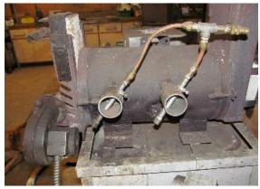
The blower is a 120V squirrel cage from the Surplus Center and is not particularly powerful. It talks to the manifold through a aluminum dryer hose. The switch on the leg controls both the main and the lateral blowers.
