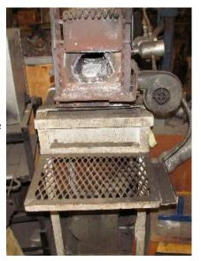
The burners are typical venturi units with 0.040 orifices and can run from 5 to 15 psi of LP pressure. They are inserted in the wall so as to project the flame towards the upper right side of the fire space.
