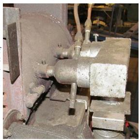
This shows the manifold removed from the burners.
